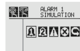
Figure 16. Alarm/Fault Simulation Menu
