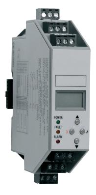
Two versions of Unipoint are available; one for mV bridge, catalytic bead type, flammable gas detector and the other for any 2 or 3 wire 4-20mA type gas detector. Each Unipoint is easily installed onto the DIN rail via a special socket (provided) that also interconnects power to adjacent units. With removable terminal connectors individual Unipoint controllers can be easily changed without disturbing other devices.
