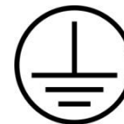
Figure 4. Equipment Earth (Ground) Point
