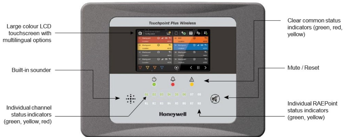
Figure 11. Touchpoint Plus Wireless Controller User Interface
