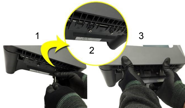
Figure 10. Undoing the Security Screws and Opening the Enclosure
