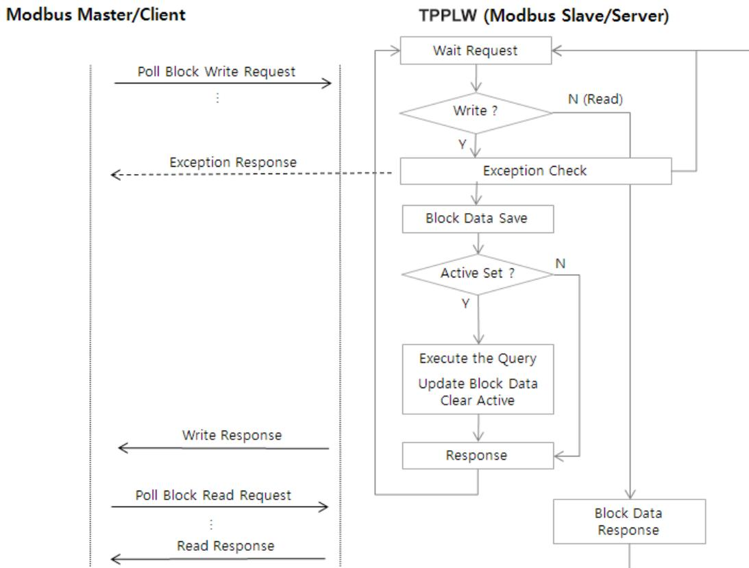
Figure 7. Modbus Query Poll Register processing procedure
