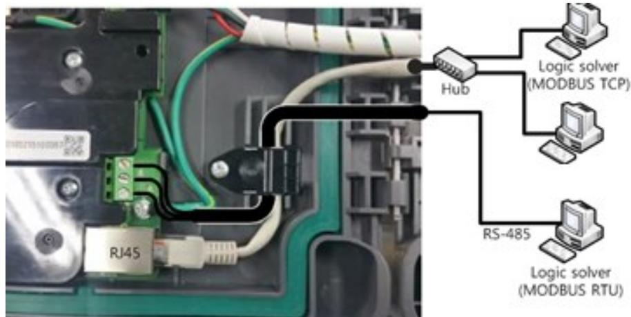
Figure 4. TPPLW Modbus TCP / RTU Client Connections
