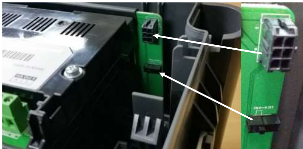
Figure 52. Battery On/Off Switch and Battery Connector
