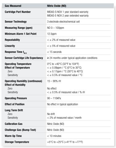
The sensor data listed is based on ideal test environment; observed performance may vary based on the actual monitoring system and the sampling conditions employed
